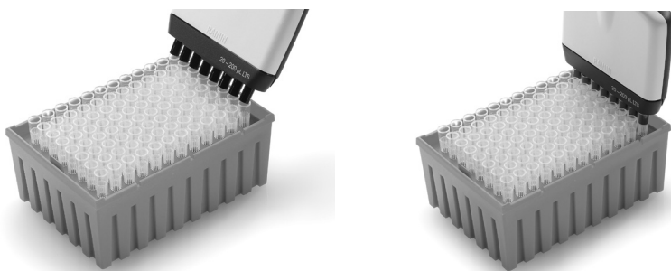
Figure 14: Mounting racked LTS Tips
