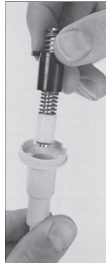
FIGURE 16.2 REMOVING THE PISTON ASSEMBLY FROM THE LIQUID END
