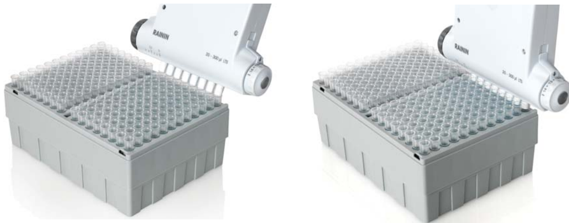
Figure 37: Mounting LTS Tips
