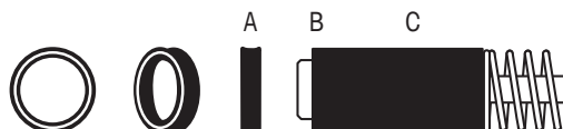
A: Seal (note open edge faces outward) B: Seal retainer C: Piston assembly
