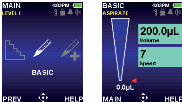
Figure 8: Basic Mode Highlighted in Level I Menu (left), Basic Mode Operating Screen (right).
