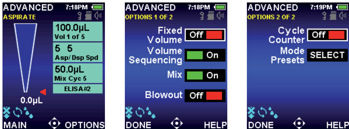
Figure 15: Options in Advanced Mode: OPTIONS Soft Key in Operating Screen (left), Options 1 of 2 (center) and Options 2 of 2 (right)
